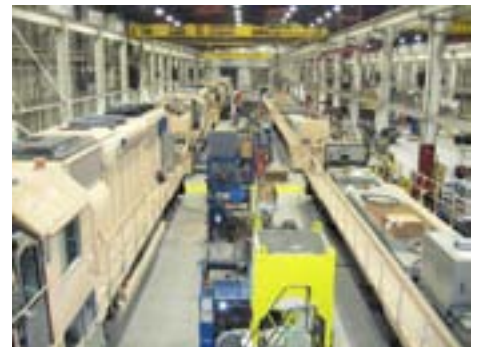
BRC’s new hump locomotive mother units, left, and three of the five slugs, right are under remanufacture at Motive Power Industries’ Boise, Idaho, plant.
